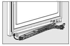
■ Insert the soft-close mechanism back into the door, starting at the right hand side.
